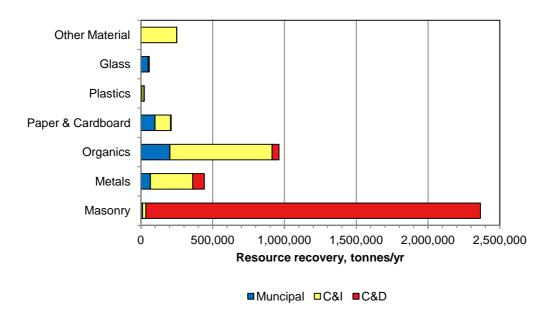
Figure 4 Sector origin of SA recovered materials according to material category (by weight, tonnes), SA 2010-11
