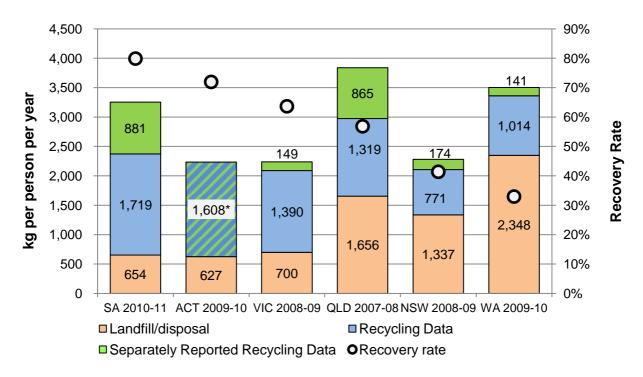
Figure 2 Comparison of reported per capita (kg/person/yr) resource recovery and landfill disposal and recovery (%) by State or Territory.<sup>6,7</sup> Note: \*ACT recycling data for 09-10 does not separately indicate soil, sand and rock from C&D data and therefore the distinction between recycling data and separately reported recycling data could not be made.
