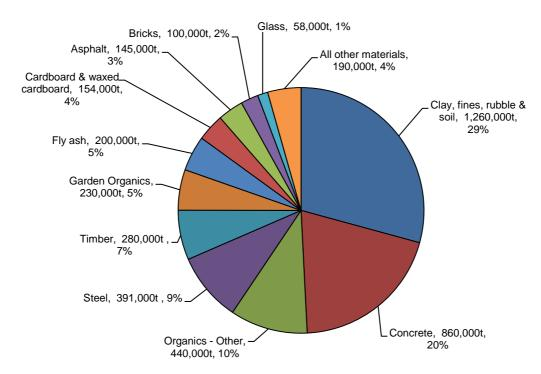
Figure 3 Composition of recovered materials (by weight, tonnes (t) and %), SA 2010-11
