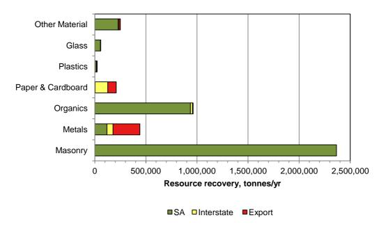
Figure 5 Destination of SA recovered materials according to material category (by weight, tonnes), SA 2010-11
